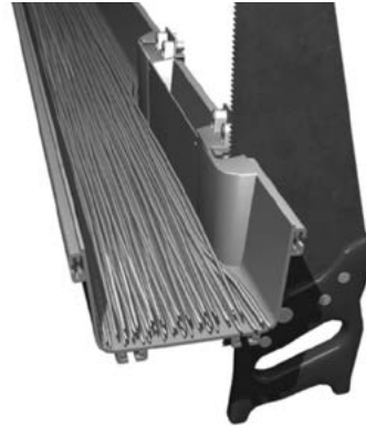
Fixture protects cables during cutting of sidewall
